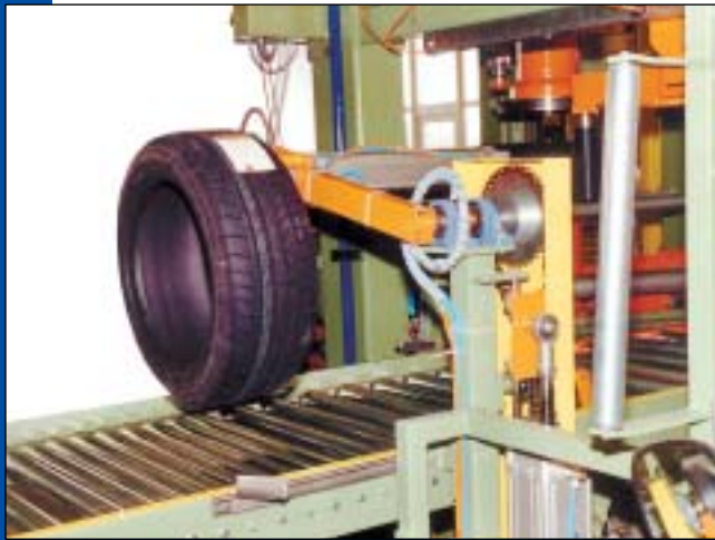
Transfer equipment for final inspection
